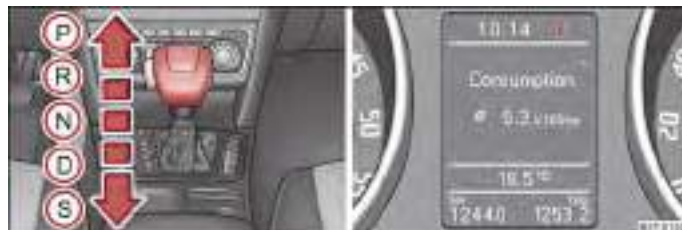
Fig. 127 Selector lever/information display: Selector lever positions
