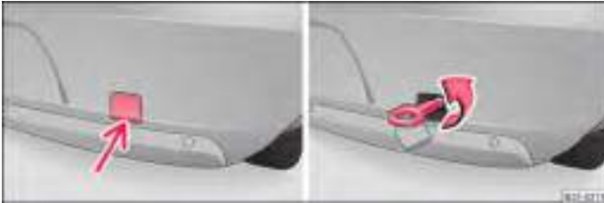
Fig. 197 Rear bumper: Removing the cover/installing the towing eye
