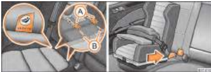
Fig. 159 Locking eyes (ISOFIX system)/the ISOFIX child seat is pushed into the mounting funnels
