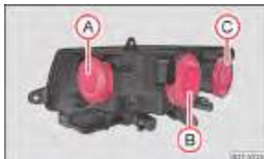
Fig. 203 Front headlight: Fitting position of the bulbs
