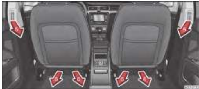
Fig. 109 Air vents at the rear
