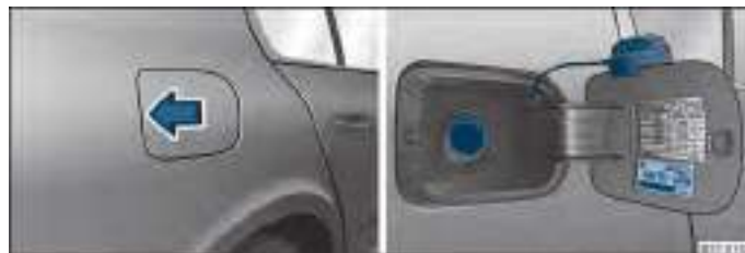
Fig. 169 Right rear side of the vehicle: Open fuel filler flap/fuel filler flap with cap unscrewed
