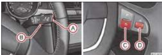
Fig. 6 Multi-functional indicator: Controls on the windshield wiper lever/controls on the multifunction steering wheel
