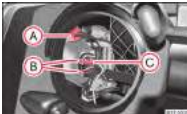
Fig. 204 Removing the bulbs for the parking and main beam light
