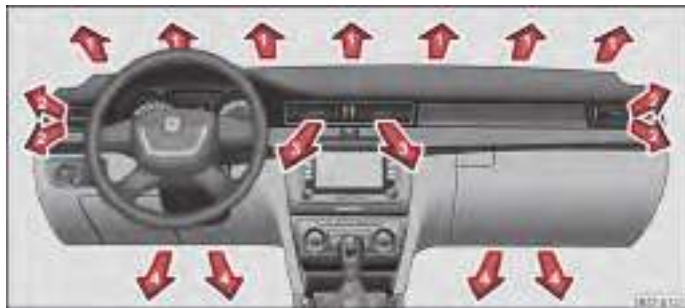
Fig. 108 Air vents at the front
