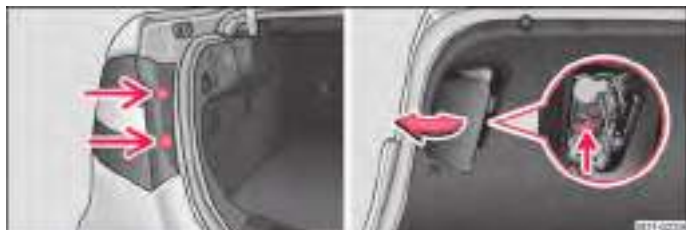
Fig. 207 Remove the outer part of the rear light unit/remove the inner part of the rear light unit
