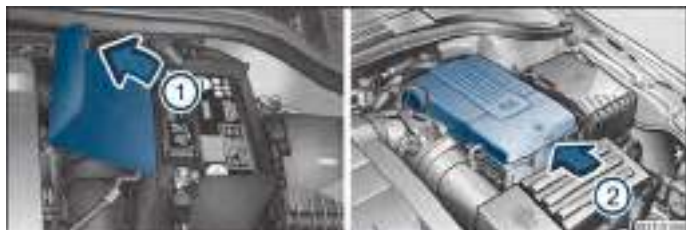
Fig. 176 Engine compartment: Polyester cover of the vehicle battery/plastic cover of the vehicle battery
