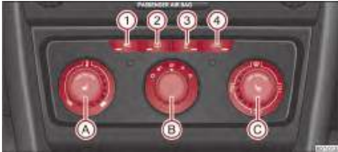
Fig. 110 The air conditioning system: Control elements
