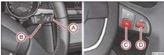
Fig. 7 Information display: Controls on the windshield wiper lever/controls on the multifunction steering wheel
