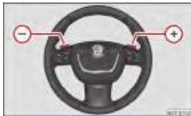
Fig. 129 Multifunction steering wheel: Manual shifting of gears
