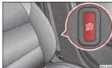
Fig. 26 Button for interior monitor and towing protection monitoring
