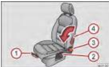
Fig. 56 Controls at seat
