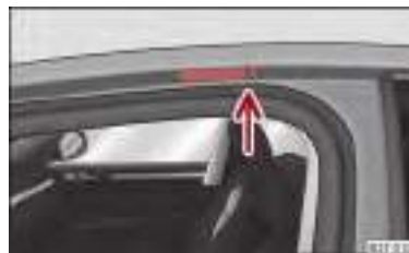
Fig. 85 Attachment points for base roof carrier
