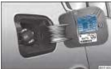
Fig. 179 An opened fuel filler flap with a tyre size and tyre inflation pressure table
