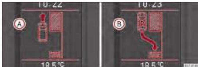
Fig. 123 Information display: the determined parking space with the information to drive on (A) and for engaging the reverse gear (B)
