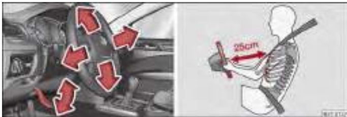
Fig. 114 Adjustable steering wheel: Lever below the steering wheel/safe distance to the steering wheel
