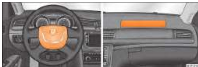
Fig. 144 Driver airbag in the steering wheel/front passenger airbag in the dash panel
