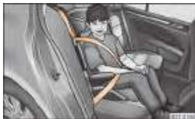
Fig. 157 Child seat in Group 2 installed on the rear seat facing the direction of travel
