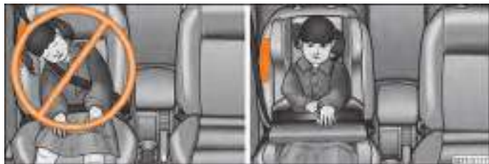
Fig. 154 Seated position of an unprotected child at risk from side airbag/Child properly protected by safety seat
