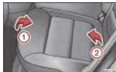
Fig. 62 Folding the seat cushion forwards
