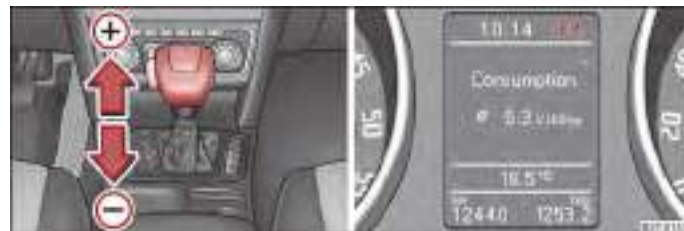
Fig. 128 Selector lever: manual shifting/information display: Manual shifting of gears
