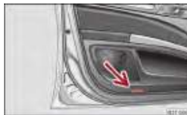
Fig. 45 Front door: Warning light
