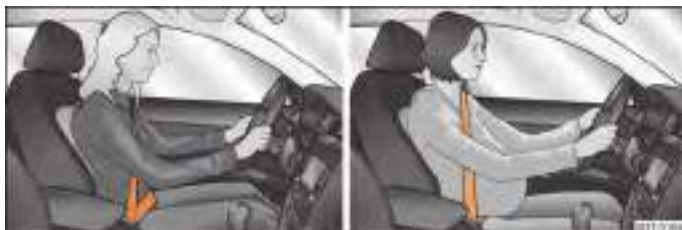
Fig. 141 Routing of belt webbing over the shoulders and the lap belt/Routing of belt webbing for an expectant mother
