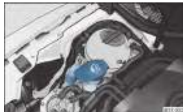
Fig. 178 Engine compartment: Windshield washer fluid reservoir
