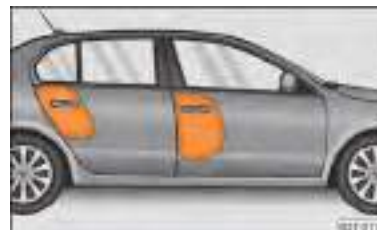
Fig. 149 Inflated side airbag
