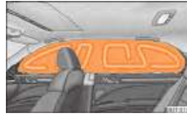
Fig. 151 Inflated head airbag
